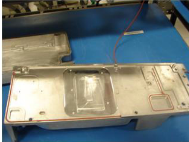
Figure 4-10 Placement of gasket on the chassis
