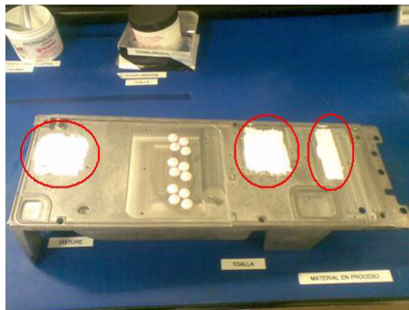
Figure 4-13 Areas to apply thermal gel
