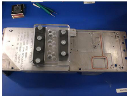
Figure 4-11 Placement of thermal gel application fixture on the chassis
